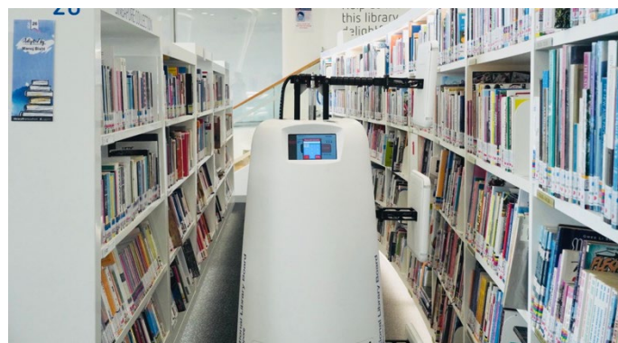
Figure 4. Shelf Reading Robot in action of scanning shelves with its multiple arms.
